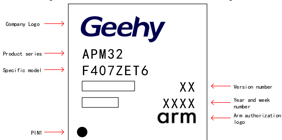
Figure 22 LQFP144 -144 Pins, 20 x20mm Schematic Diagram
